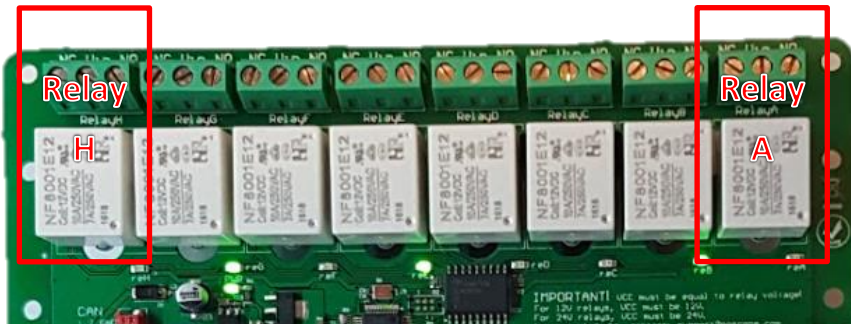
Figure 3: Relay naming - relay outputs are marked with letters A to H in order as indicated
